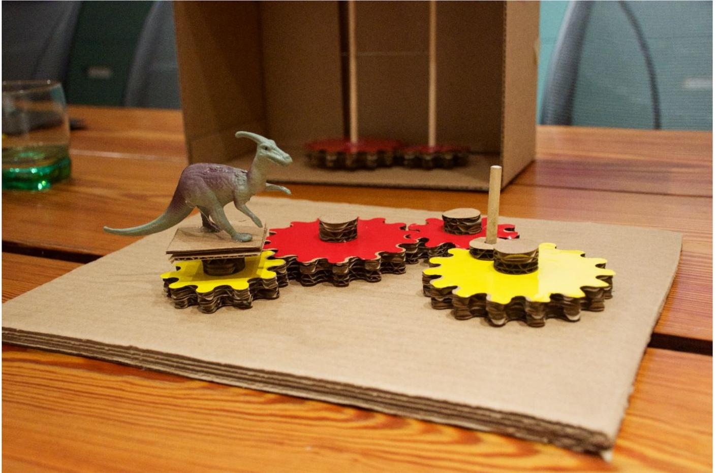
Deer Isle-Stonington Elementary School students used computer software and laser cutters to design cardboard automata, gear-driven moving mechanical devices which helped them understand the transfer of energy between components. PHOTO BY DAVID ROZA
